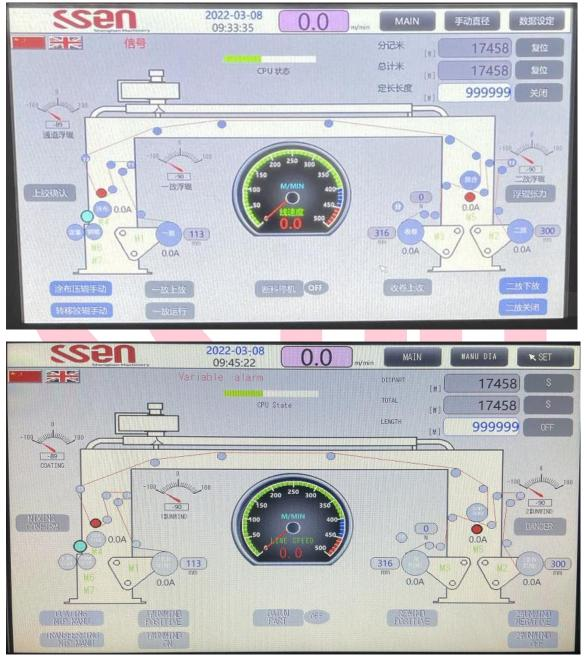
\* Dispart: Length of each rewinding reel material; S(reset): clear the meters number.
