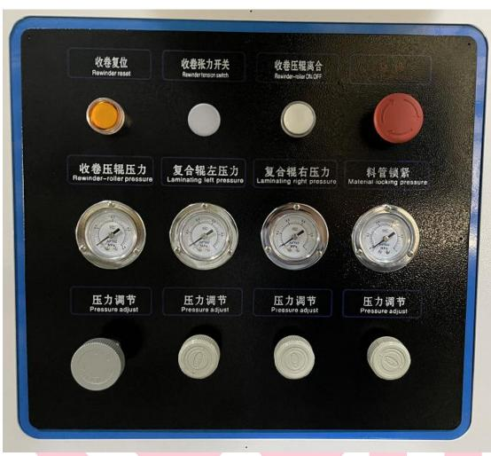
Rewinder reset: Reset the rewinding reel diameters. Rewinder-roller ON/OFF: Control the rewinding press roller clutch and rewinding tension switch.
