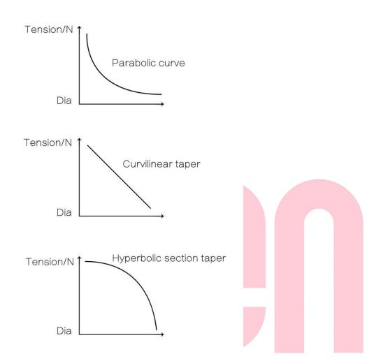
**\* Tension:** Initial tension of rewinding core.
