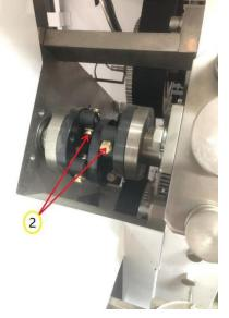
Point (1): fix the bearing with the plug for unwinds and rewind parts, and add 1# grease (once a month).
