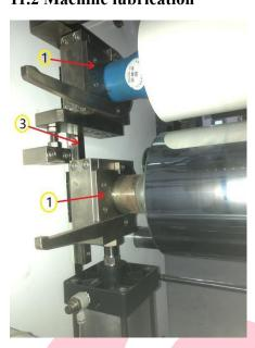
Point (1), Remove the bearing cover of the laminate press roll and backup press roll, and add 1# grease (once a month).
