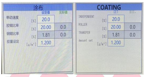
**\* Independent:** Refers to the idling speed of the metering roller(R2), transfer rubber roller(R3), and coating roller(R4) at the same time.
