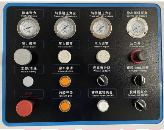
Window Up/Down: Control the up and down of observe window.
