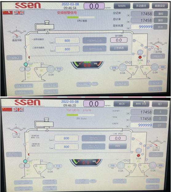
1#Unwind manual dia.: The initial diameter of the unwinding material must be manually input and reset before the machine is started.
